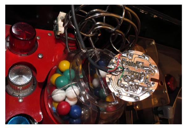
Pull the wire taught and out by the metal circle of the gall guide and tie it there with the black ty-wrap. Cut off the excess wrap. The cable must be held tight against the top of the ball hole in the machine so the ball does not get stuck when trying to enter.
