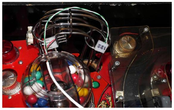
Install the diverter with the cable on the left side. The dazzler board will fit into the cutout of the diverter with the cable exiting in a notch by the slot. The dazzler board will fit down in the machine flat on the diverter and the side dividers.
