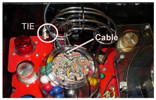
Install the cover back on the gumball machine. Route the cable over the back board and up into the backbox..
