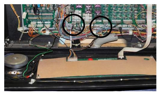
Unplug the plug on J116 and plug the dazzler plug with pins sticking out the back onto J116. Then re-connect the plug that was there on the dazzler plug J116. There are only 3 pins. Line the bodies up. Plug 122 onto J122 right end. The white wire will be to the left as shown below.
