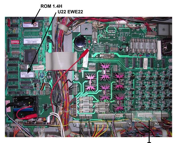
Plug the yellow wire onto J125 only if ROM 1.4H and EWE22 is installed on the CPU board. It has NO effect with 1.3X and below ROMs.
