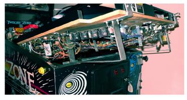
Rotate the yellow handle in the coin door to the left releasing the cover glass lock bar. Lift it off and close the coin door. Slide the cover glass off and set it safely to the side. Pull the ball shooter out about an inch with your right hand an lift up on the playfield arch with your left hand to clear the plunger. Now use both hands to lift the playfield up and pull it onto the support rails.
