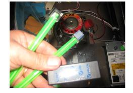
Step 4 - The attach the power supply box, and lights under the machine using provided velcro as shown. Horizontal in the front and vertical in the rear.
