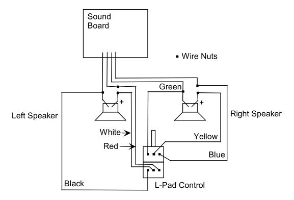
Connect the Black and Green wires to the negative (-) speaker (black) wires by removing about 3/4" of the insulation (no need to cut the wire) and twist the Black or Green wire together with the bared wire using a wire nut. Cut the positive (+) speaker wire 2" or 3" from the speaker terminal and attach the Red, White, Blue, and Yellow wires as shown.
