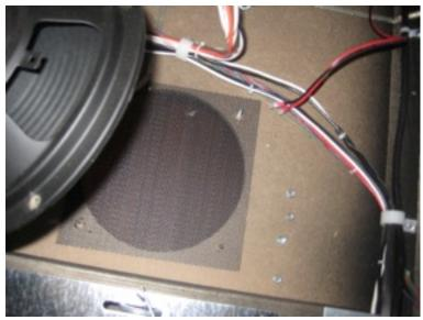
Install the subwoofer on the studs being careful not to damage the cone or surround. Install the nuts and snug them. Plug the leads from the backbox onto the subwoofer board. The Red lead goes on the lug marked +. Black to the "-". If there is a ground wire for the speaker frame, reconnect it.
