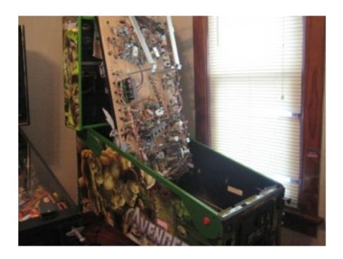
Carefully remove the base cabinet speaker. You can desolder or clip the wires and take it out of the cabinet.
