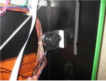
Unplug the speaker connector from the sound board and plug the wire with the plug from the L-Pad into it. You can leave the old wiring in place. Connect the 4 pin (SWTR-4, SWTR-4-12, SWTR-4LE) or 5 pin (STWR-4A) plug onto the sound board. Observe the locking tabs for proper connection. Route the long wire into the base cabinet for the subwoofer and connect the lighter gauge speaker wires to the backbox speakers. The longer of the two goes to the left speaker. Reinstall the speaker panel only.
