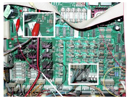
Mount the fork lug that is on the black wire under a mounting screw as shown. Clip the red alligator on TP1 for 12 volts as shown. Lower the TV down into the base cabinet carefully and push all the extra cable down with it. Close up the backbox reversing the steps.
